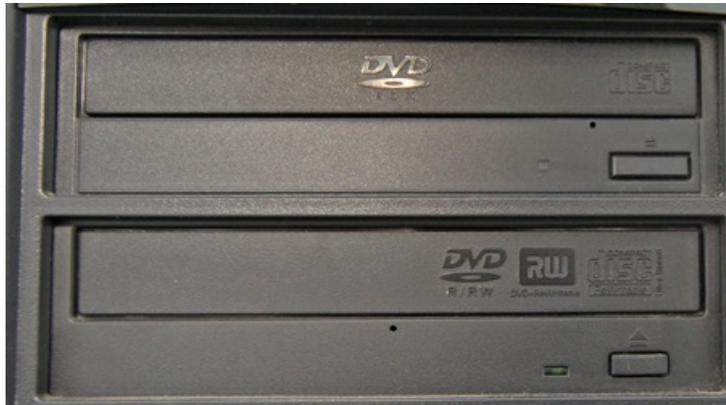
The PC above has two drives: a DVD reader at the top, and a combined DVD/CD reader/writer underneath. These are actually drawer-like trays, into which a DVD or CD is laid and then the tray is closed.
