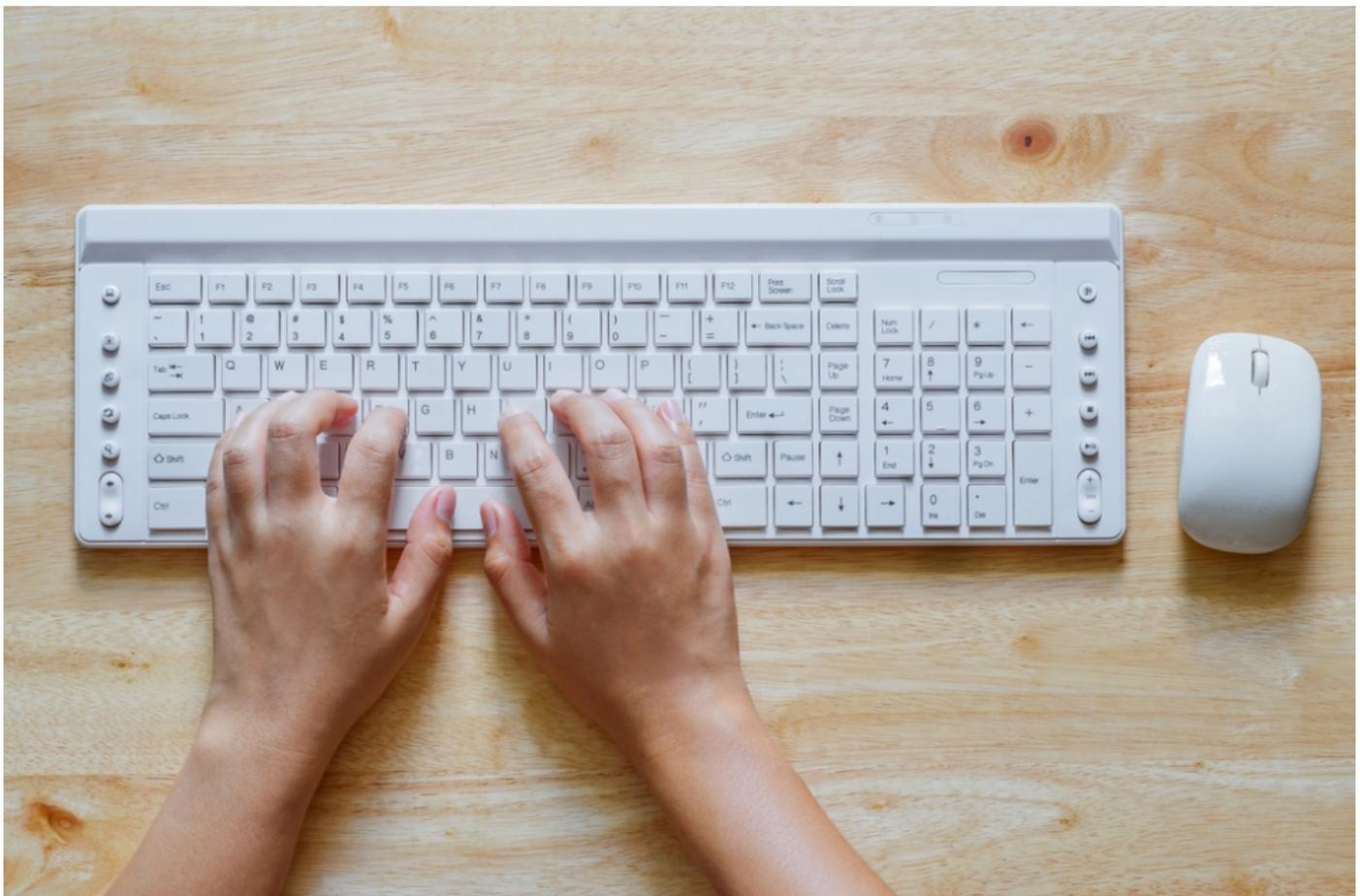
The most common kind of keyboard is referred to as a 'QWERTY' keyboard after the keys on the top row of letters. It was invented by C L Scholes in the 1860s when he was working out the best place to put the keys on a manual typewriter.
