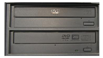
The PC above has two drives: a DVD reader at the top, and a combined DVD/CD reader/writer underneath. These are actually drawer-like trays, into which a DVD or CD is laid and then the tray is closed.
